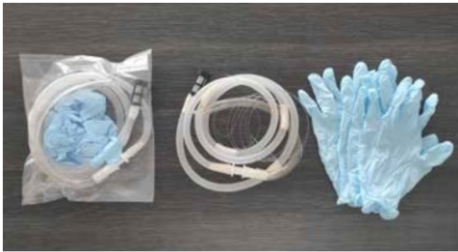
Figure 16 : VigiDNA® sampling kits. On left: Tube with an inlet filter and disposable gloves. On right: Filtration capsules, stoppers and conservation buffer (© SPYGEN)
