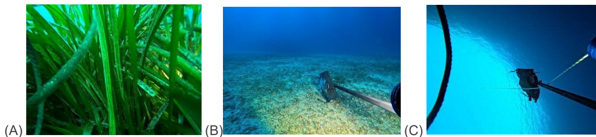
Figure 13: Examples of settle conditions: (A) bad visibility (0, we don't see the bait), (B) soft bottom and settle condition ok, (C) bad settle condition (rig towards the surface) ©Lauriane Guérin, OFB-PatriNat
