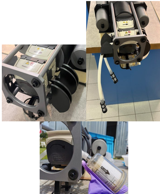
Figure 19 : Installation of the tube and the filter on the pump
