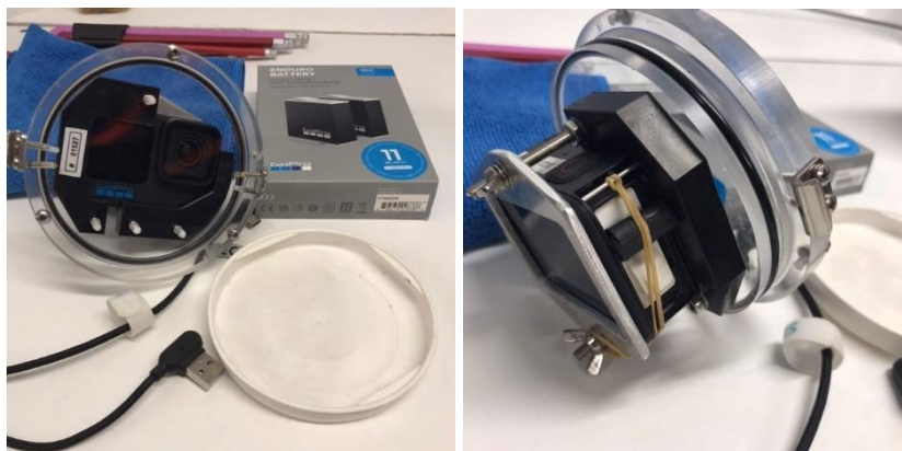
Figure 22: (Left) Front view of GoPro 11 mounted on the camera port, with the plastic lid and extra battery pack. (Right) Side view of camera port, with the cover removed to allow the cable connection (cable outlet for the model is located under the battery (white) © Havforskningsinstituttet
