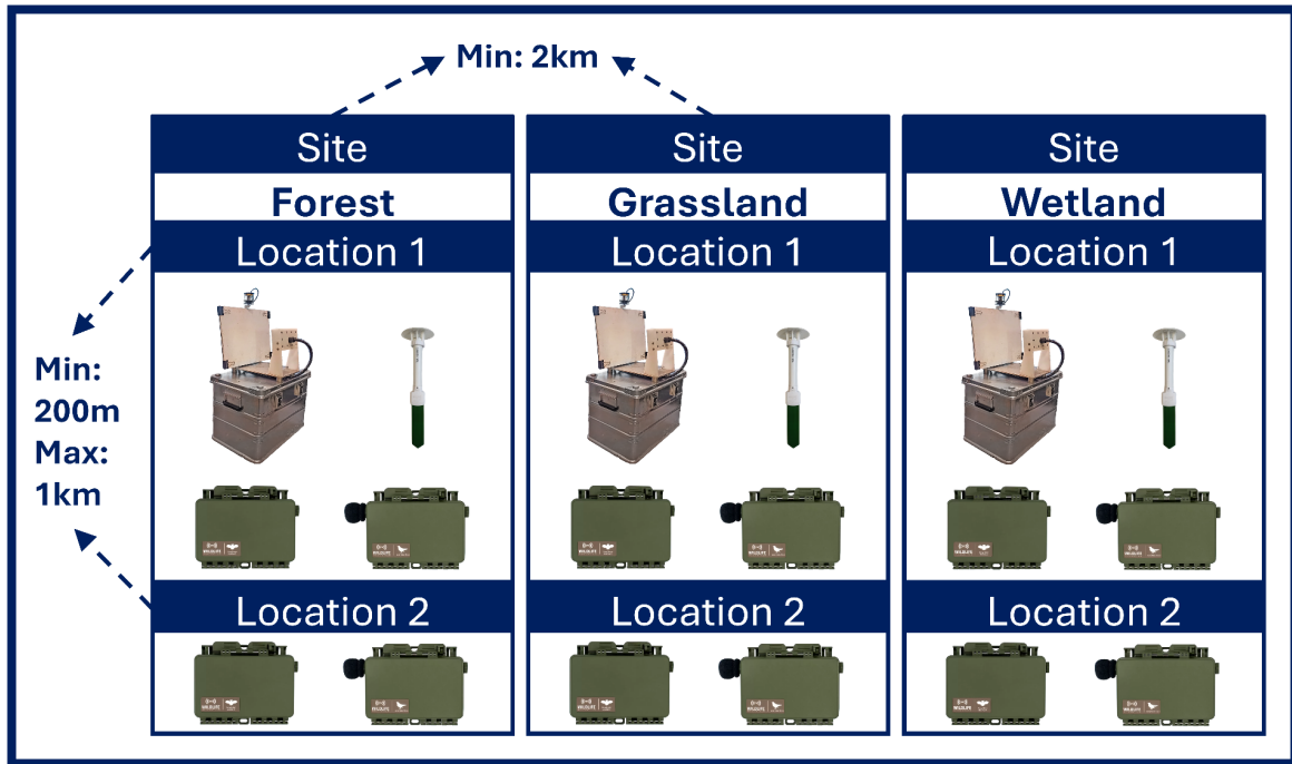
Figure 1. Overall design of ABMS sampling with AMI devices, Song Meter devices and TMS-4 climate loggers. Up to two locations were sampled at sites associated with three broad habitat types: forest, grassland and wetland.
