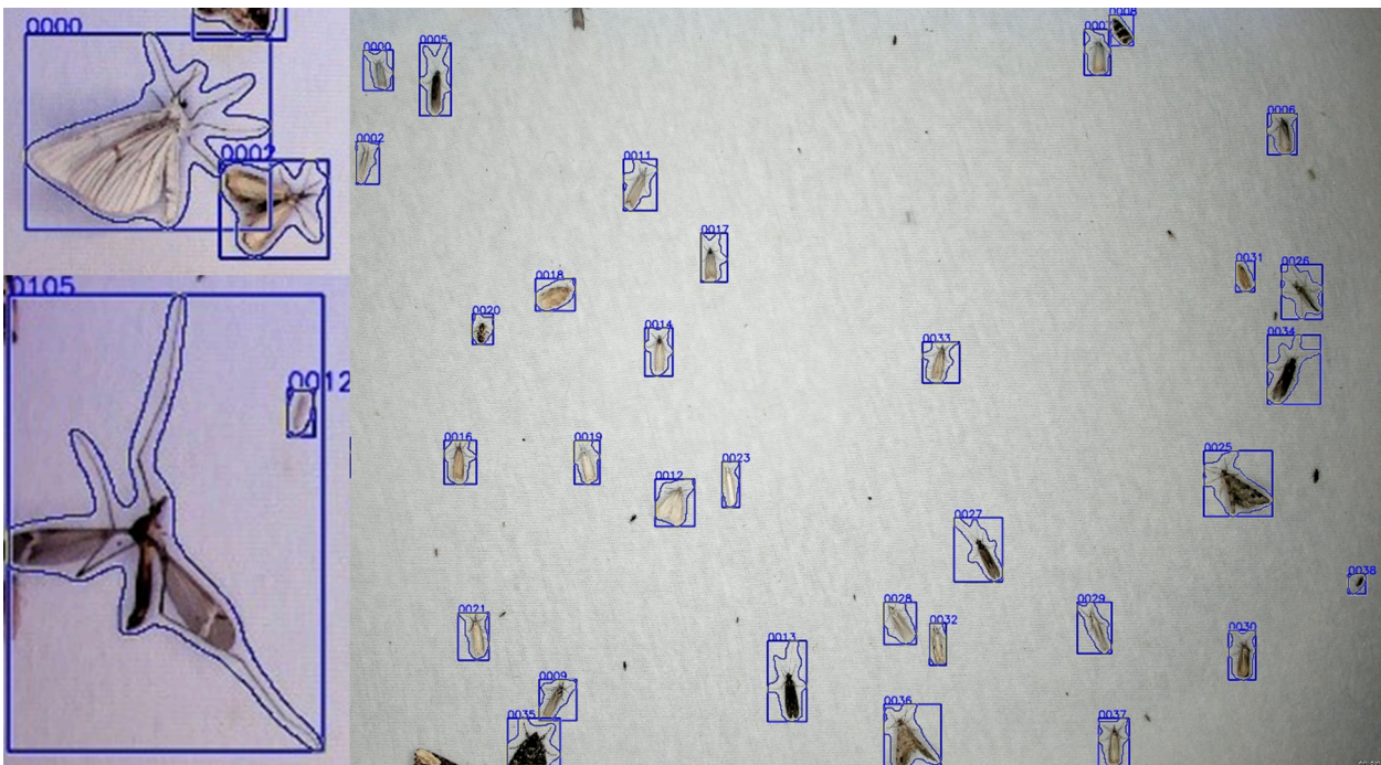
Figure 3: Example of an image recorded with the AMI trap. The new localisation model for AMI trap images draws a segmentation polygon as well as the rectangular bounding box around each detected animal. These are also shown in the main image as well as in two insets of zoomed in details from a similar image highlighting details for individual animals (Svenning et al., unpublished data).
