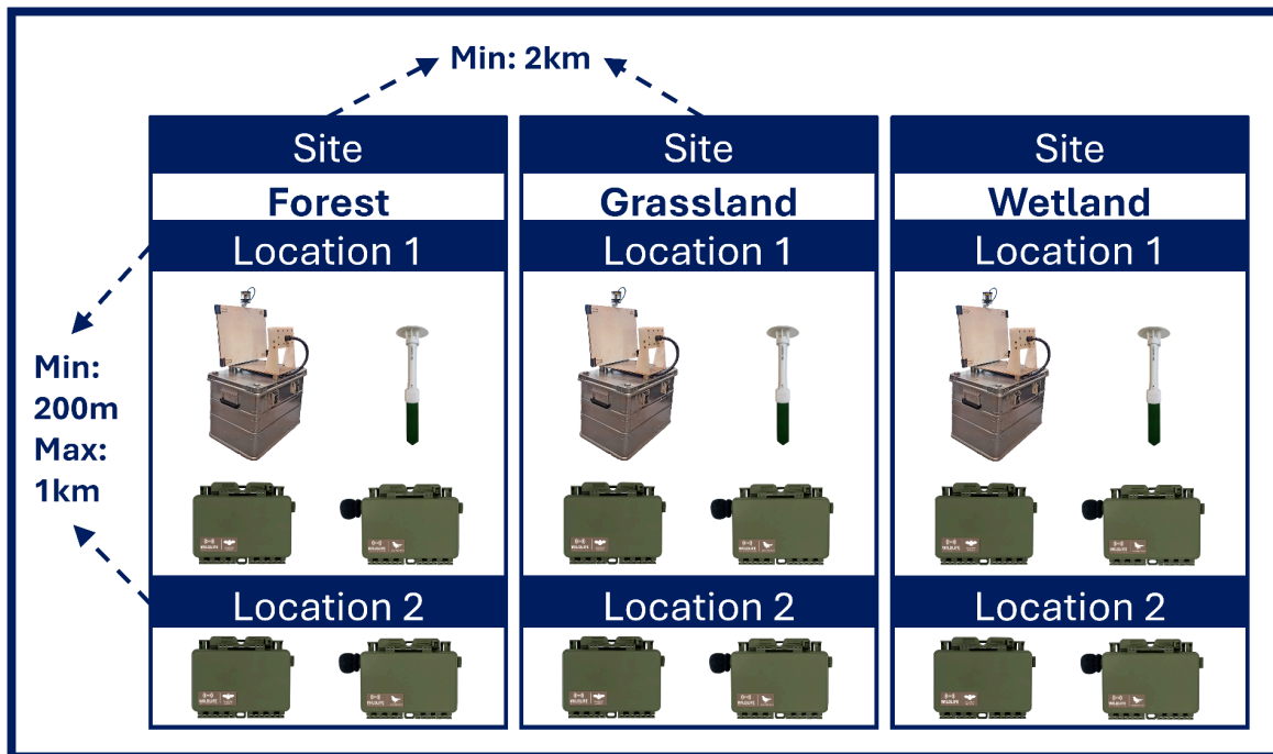
Figure 1. Overall design of ABMS sampling with AMI devices, Song Meter devices and TMS-4 climate loggers. Up to two locations were sampled at sites associated with three broad habitat types: forest, grassland and wetland.
