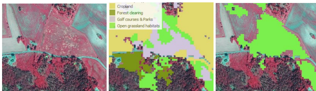
A4_Fig 7 Aerial photograph (left), RF classification after sieve (middle), grassland mask extracted from the classification, after adjustments made for overpredicted urban parks, golf courses, and grassland.
