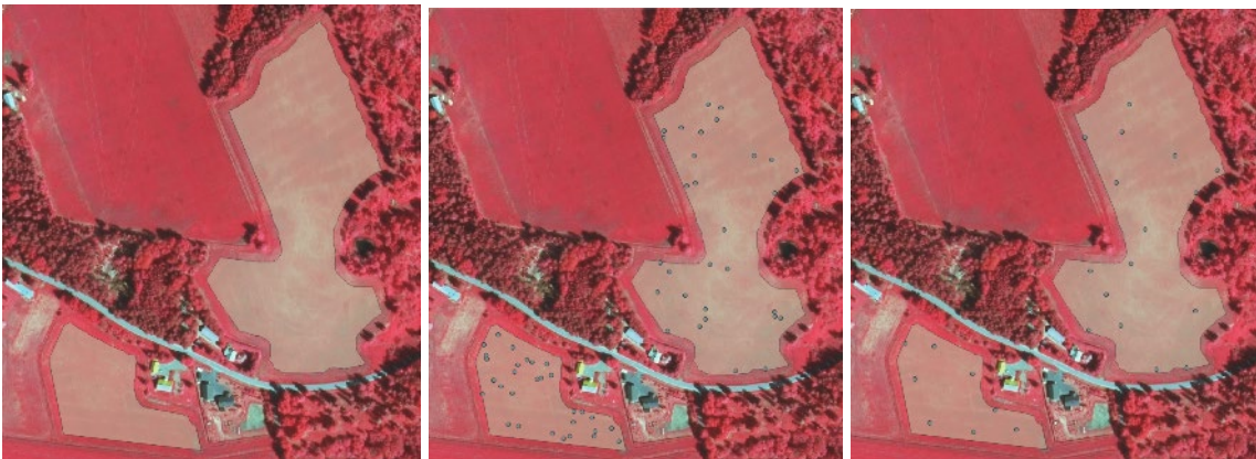
A4_Fig 2 Illustration of the stratified point sampling. Left: two reference polygons with edges (10 m) removed, middle: random points, right: remaining points after removing too close ones.
