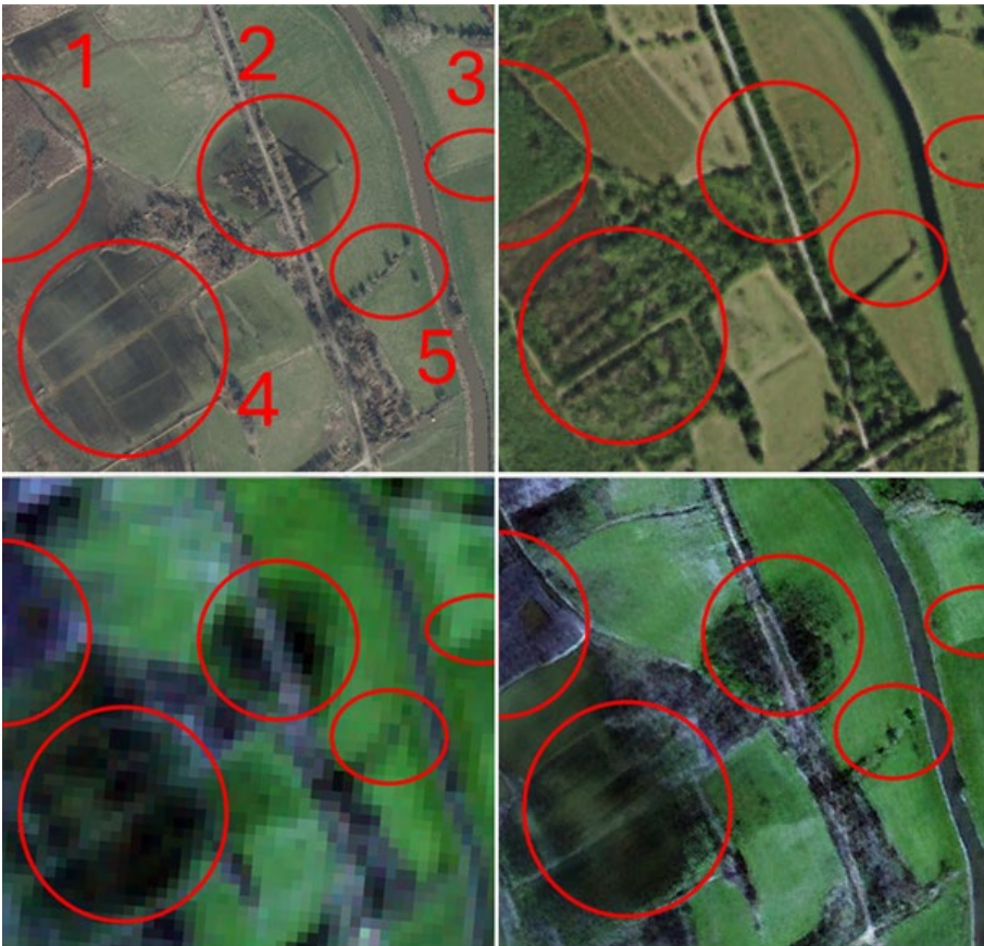
A7_Fig 2 Example demonstrating the distinguishability of landscape features including a reedbed (1), an inundated forest area (2), a river (3), an inundated open area (4), and a tree line (5) visualized in an ortho photo (t.l.), Sentinel-2 scene (b.l.), Satlas image (t.r.), and S2DR3 image (b.r.)
