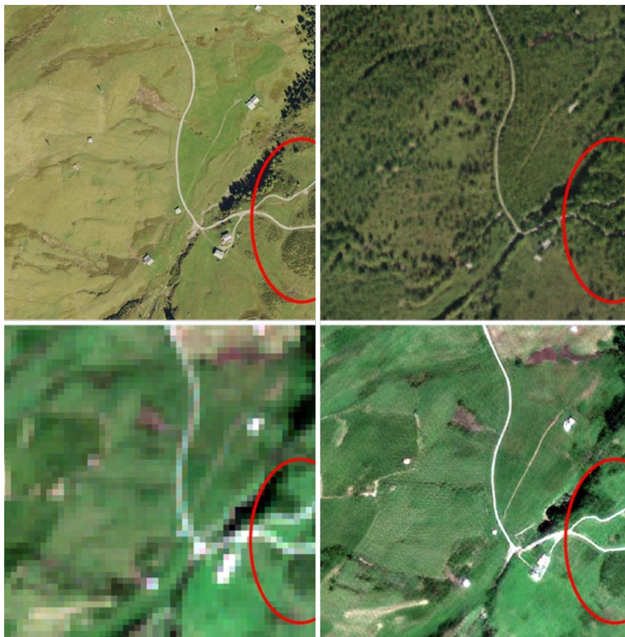
A7_Fig 3 Example demonstrating tree-like ‘hallucinations’ of the Satlas model (t.r.) making e.g., the detection of Rhododendron shrubs (circled) more difficult than in the S2DR3 image (b.r.). Orthophoto (t.l.) and Sentinel-2 scene (b.l.) included for reference.
