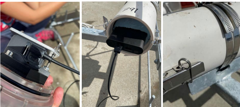
Figure 21: Camera housing details: (Left) Side view of GoPro camera with angled cable connected to the power bank (Middle) Side view of underwater housing with safety clip (Right) Behind the camera port is the powerbank that is secured in a custom-made foam holder © Havforskningsinstituttet
