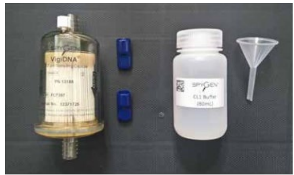
Figure 16 : VigiDNA® sampling kits. On left: Tube with an inlet filter and disposable gloves. On right: Filtration capsules, stoppers and conservation buffer (© SPYGEN)
