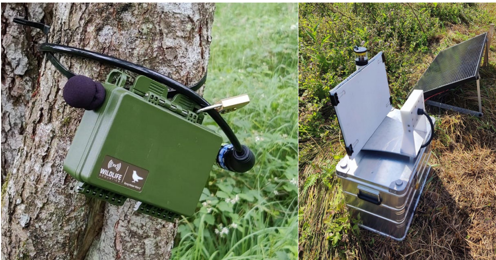
Left: A Song Meter Mini 2 deployed in Denmark. Right: An AMI trap deployed in Belgium. Photo credit Jamie Alison (left) and Lucia Manzanares (right).
