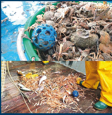
The Metaprobe (passive eDNA collector) will be used by fishers to easily collect eDNA during fishing operations and map the marine biodiversity
