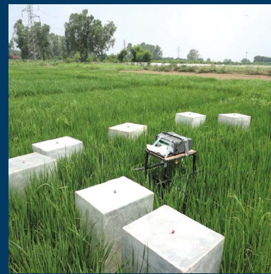
Measurement of GHG fluxes in the paddy fields using a Photoacoustic Multi-gas Monitor
