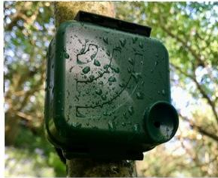
Automated moth camera trap
