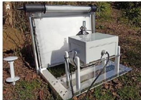
Automated moth camera trap
