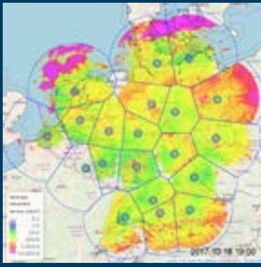
Composite image of vertically integrated density of birds extracted from weather radars in Europe on a night of intense bird migration (18-10-2017 19:00 UTC). Green - orange reflectivity due to birds.
