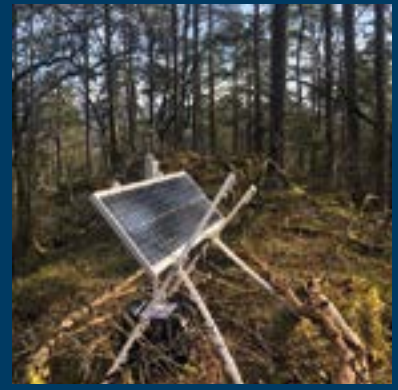
Acoustic recorder device connected to a solar panel in a forest.
