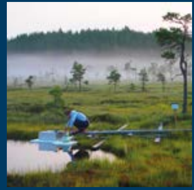
Methane measurements from a Southern Boreal bog with a floating chamber system.
