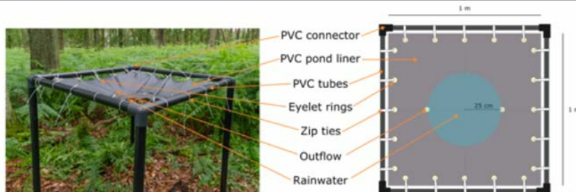
Supplementary Figure 1: Schematic overview of the rain sampler prototype.
