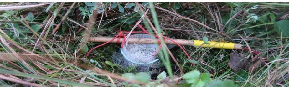
Ingrowth cores (0-50 cm), 3 per plot, Filled with sand/granulate (tested)
